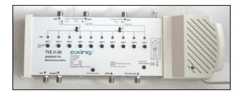
TVS 31-00 is a multi-band channel amplifier designed for digital MATV systems. It is equipped with 7 selective UHF, 3 selective VHF filters and FM amplifier.
