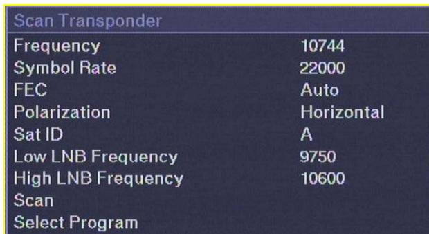
If channels are not stored, write the parameters of transponder and press “Scan”.
