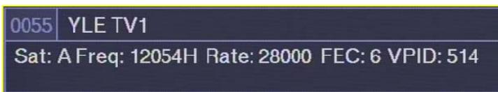
Next program info for channel previously selected is displayed and the channel opened, if possible. Info shows satellite number i.e. DiSEqC switch control, transponder frequency, data rate, FEC and channel video PID number.
