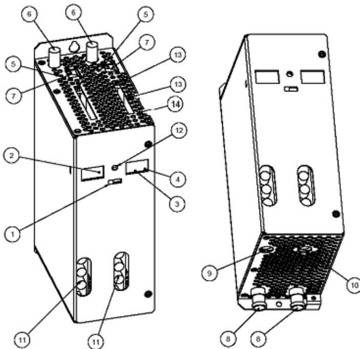
1. Control switch to program channel 1 (left) or channel 2 (right). The switch must be set to middle position when programming is ready
